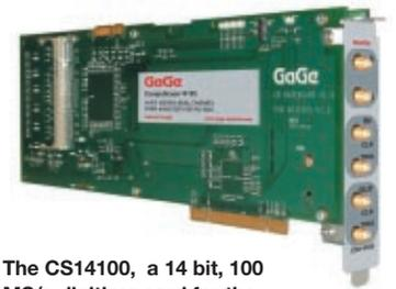
The CS14100, a 14 bit, 100 MS/s digitizer card for the PCI bus can monitor signals onboard an aircraft
